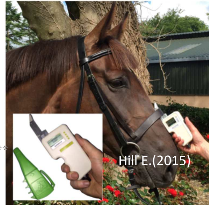
Fig 4. Digital tightness gauge, version 4 (DTGv4) deployed at a frontal site—nasal plane. Inset shows a close up of the gauge along side the ISES taper gauge.
